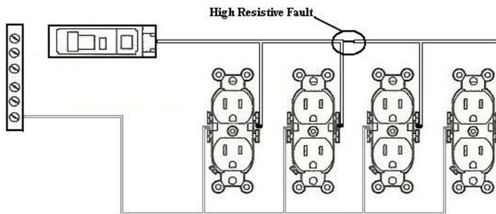
*In this example there is a High Resistance Fault between the 2<sup>nd</sup> and 3<sup>rd</sup> receptacle. The Voltage drop increased from the 2<sup>nd</sup> to the 3<sup>rd</sup>. The high resistance was identified as a poor connection between the two devices.*
