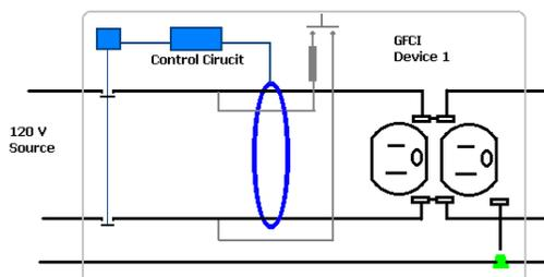
*A GFCI is a device with a built in circuit to detect leakage current to ground on the load side of the device. When the GFCI detects leakage current to ground, it will interrupt power to the load side of the device, halting a hazardous ground fault condition.*
