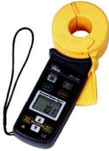
*A ground resistance clamp meter enables electricians to measure the resistance of the ground electrode in a fraction of the time required using the traditional three-point fall of potential test.*
