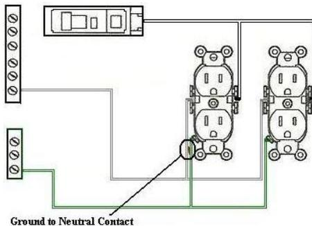
*SureTest® Circuit Analyzer can detect a false ground condition within 15 feet of a receptacle under test or within 15 feet of the panel.*
