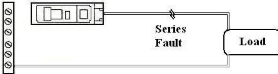
**Glowing Contact, or High Resistance Series Arcing Fault**<sup>3</sup> is defined as the abnormally high resistance in a wire, wire termination, wire splice or any type of connection, resulting in reduced current flow and excessive heat at the fault.
