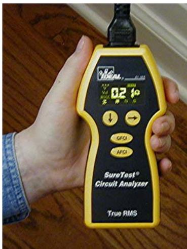
*the IDEAL SureTest® can measure the resistance of the Line, Neutral, and Ground conductors. This can be very helpful when trying to locate a high resistance fault in a branch circuit.*
